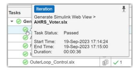
For each task iteration, the build system runs the InputQueries to find the inputs for that specific task iteration. For each input, the build system runs the InputDependencyQuery to find any additional dependencies that can affect whether task results are up-to-date. The task inputs appear under Inputs and the additional dependencies appear under Dependencies in the I/O column in Process Advisor.
