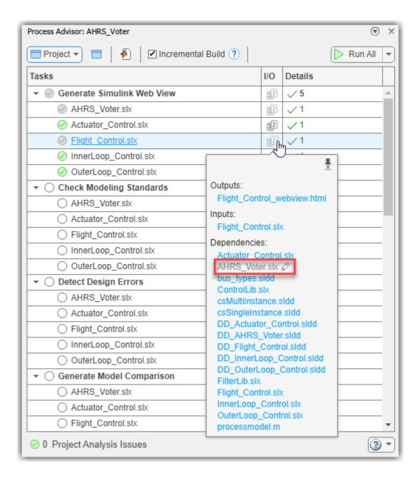
Re-run the **Generate Simulink Web View** task to get updated task results. Point to the **Generate Simulink Web View** task and click the run button  $\triangleright$ .
