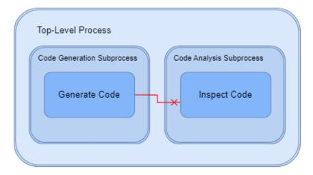
If you try to have a code analysis task in one subprocess depend on a code generation task in another subprocess, Process Advisor generates an error like: Invalid dependency between Task 'padv.builtin.task.RunCodeInspection' and 'padv.builtin.task.GenerateCode'. Make sure 'padv.builtin.task.GenerateCode' exists in the current process and that the dependency does not cross any subprocess boundaries.
