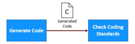
To specify that the generated code output by **Generate Code** task is the input for the **Check Coding Standards** task, the **Check Coding Standards** task uses the built-in query padv.builtin.query.GetOutputsOfDependentTask to find the outputs from the **Generate Code** task:
